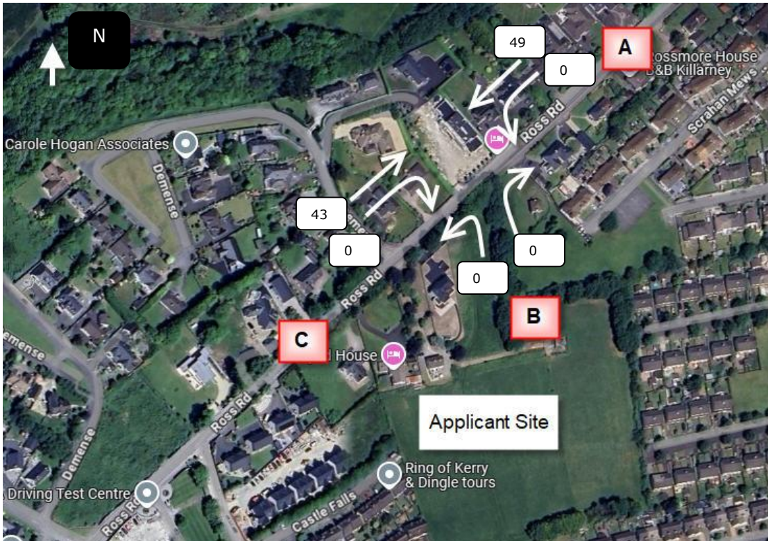
Figure 4.4: Current AM Turning Counts for Junction A
